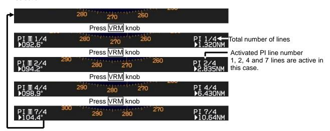
**2** While activated, the bearing and range are shown at the lower left and lower right of the display, respectively.
