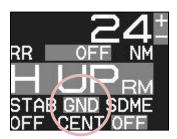
When SDME or EPFS is not available for any reason, it is possible to get the speed over ground by setting reference target.
