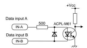
Serial data input circuit
