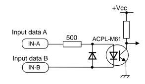
Serial data input circuit
