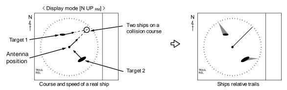
Target 1, whose trail is overlapping the EBL, is a dangerous target while the Target 2 is not. If trail setting is six minutes, and if the trail length is equal to the distance between the antenna position and Target 1, then the collision will occur after six minutes.
