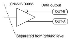
Serial data output circuit
