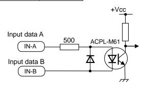
Serial data input circuit
