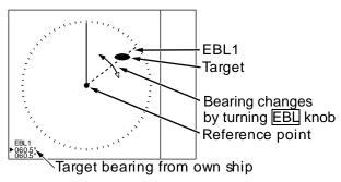
Note: Turning EBL knob (while pressing it) changes the bearing quickly.
