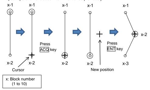
**6** When add operation is completed, press MENU key, numerical marks on the display will disappear, and nav line cross alarm will be activated.
