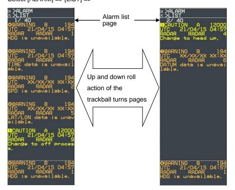
Alarm goes off automatically when cause of alarm disappears.
