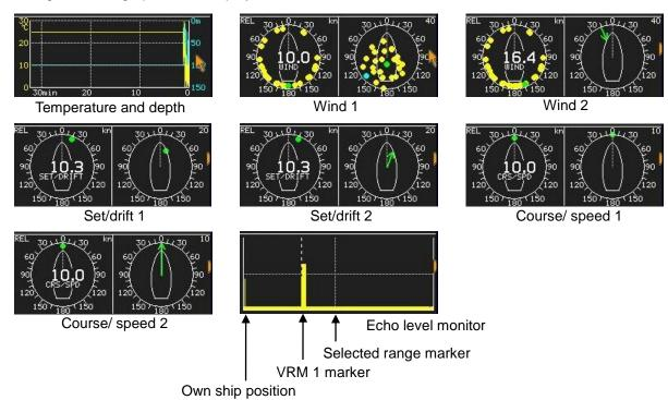
It is necessary to input MTW sentence to display water temperature.
