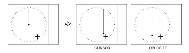
Note: When CCRP is selected for the reference positon, there is possibility that CCRP is located outside of 90% echo image area at OFF CENTER function in short range.
