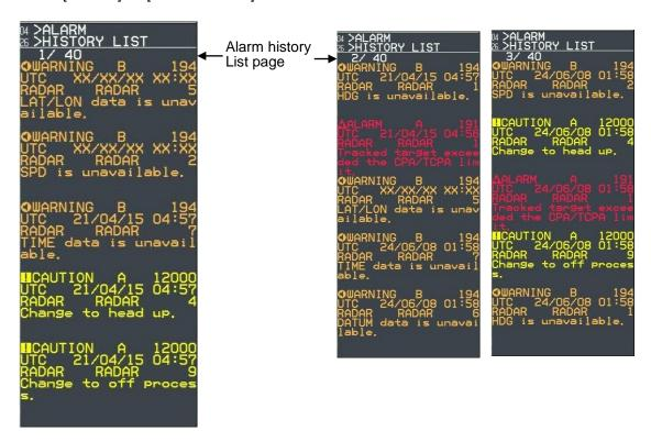
Maximum number of alarms which can be displayed is 200. Alarms in excess of 200 are deleted. The up and down roll action of the trackball turns 40 pages.
