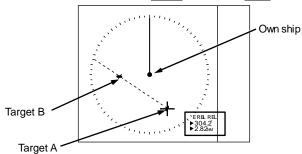
**3** Pressing ENT key (while pressing OFF key) returns cursor to the reference point position. Therefore, it is possible to measure the distance/bearing from the reference point position.
