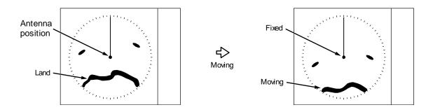
**True motion (TM)**: The antenna position on the display moves according to its speed and tidal current.
