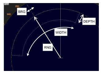
Note: If the echo alarm area is set in the whole circumference, [WIDTH] needs to be set the  $0.0^{\circ}$  or  $360.0^{\circ}$ .
