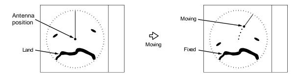
N-UP or C-UP TM mode is selected, own ship position moves to opposite side of heading direction, and begins to show the true motion image. When own ship position reaches center of the range scale, own ship position is to reset to the course over water or to the opposite direction of the course over ground.
