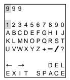
2 Select each letter one by one and press ENT key after each letter, when finished select [EXIT] and press ENT key.
