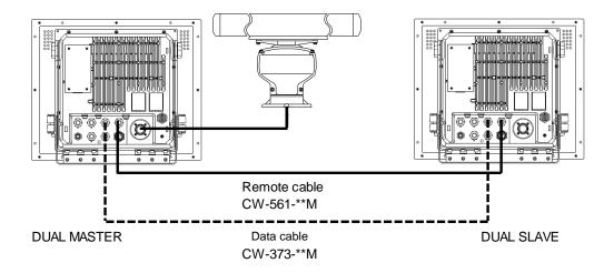
CROSS: In this status, there are two radars to which each antenna is connected. In this status, the antenna that is not connected to its own radar is used.
