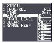
[TRAIL LEVEL]: This is to set up echo level of trail to be recorded.
