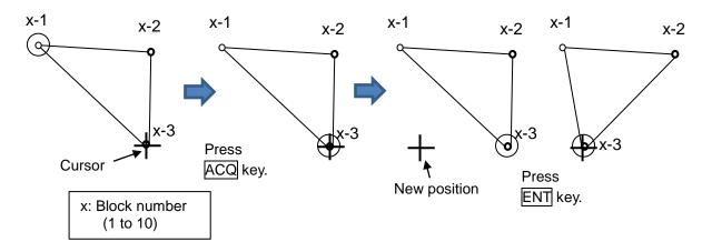
**6** When move operation is completed, press MENU key, numerical marks on the display will disappear, and map area alarm function will be active.
