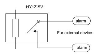
Note: Alarm contact will close in case of failure.
