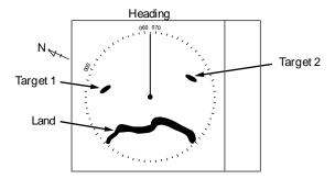
When heading signal is connected, H UP works by stabilized mode. (STAB H UP)
