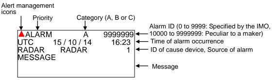
In case of unacknowledged alarm, icon and ALARM of priority will be flashing, and 3 short audible signals will be repeating every 7 sec.
