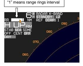
Note: When [NAV TOOL] => [BRG TRUE / REL] => [TRUE] is selected, 0° of the range rings indicates North direction. While, when [REL] is selected it indicates heading direction.
