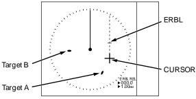
**2** By moving cursor to target A, measurement of distance and bearing from target A to target B can be obtained by using VRM knob and EBL knob.
