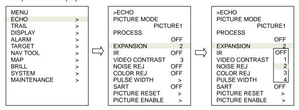
Note: "Menu" setup value is stored in the non-volatile memory inside the radar. Therefore, no setup operation is required after power is turned on.
