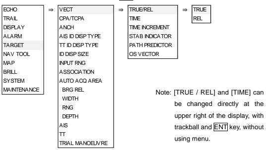
2 In addition, there are [TIME], [TIME INCREMENT], [STAB INDICATOR], [PATH INDICATOR] and [OS VECTOR] setups.
